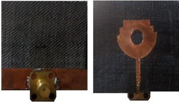
Fig. 8: Hardware of Proposed Antenna (A) Front View (B) Back View.
