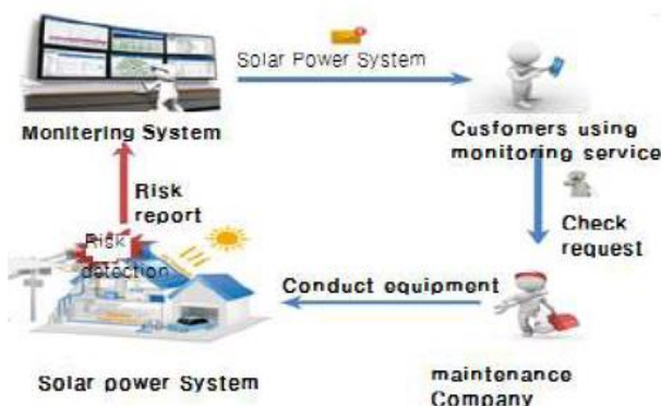
Fig. 5: Solar Monitoring System Based on Iot Platform.
