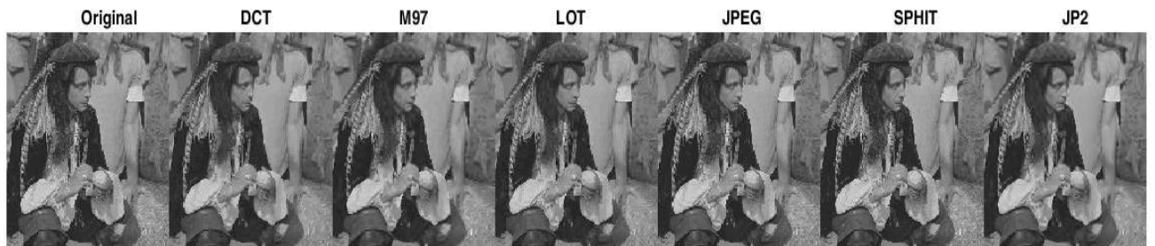
Fig. 4: To the left we see the original image of man and to the right the image is compressed using different algorithms such as DCT, M97, LOT, JPEG, SPIHT and JP2K.
