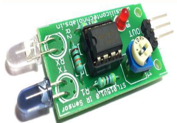
Fig. 5: IR Proximity Sensor.
