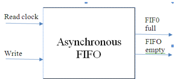
Fig. 2: Clock Domains in Asynchronous FIFO.
