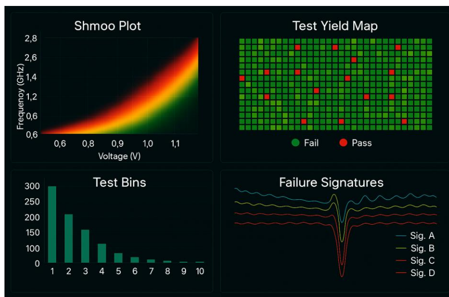
Fig. 1: Presents A Real-Time Dashboard Image That Aligns Shmoo Plots, Yield Maps, And Fail Signatures with Test Bins.
