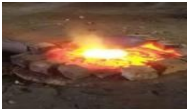
Fig. 1: LTB in Molten State in Pit Furnace.
