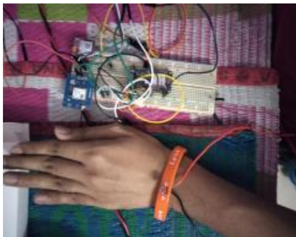
Fig. 5: Smart Wrist-Band for Emergency Communication.
