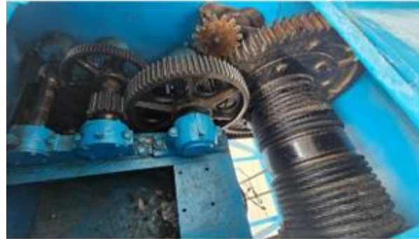
Fig. 3: Spur Gear Assembly with Rope Assembly.
