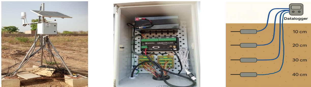
Fig. 1: Field Instrumentation Used for Soil and Meteorological Data Acquisition at the Tanghin Experimental Site (Saaba, Burkina Faso). (Left) The ClimaVUE50 Autonomous Weather Station, mounted on A Metallic Frame and powered by A Solar Panel System, Records Key Atmospheric Variables. (Center) Internal View of the Control Unit Containing the CR350-CELL215 Datalogger and Wiring for Real-Time Data Transmission. (Right) Cross-Sectional Schematic of the Sensor Layout Showing TERS21 Probes Deployed At 10, 20, 30, and 40 Cm Depths, Each Individually Connected to the Datalogger.
