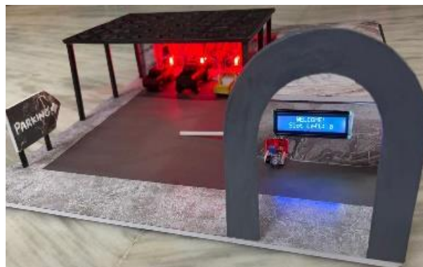
Fig. 5: Physical Model Showing Full Parking Slots with Red LED Indication.
