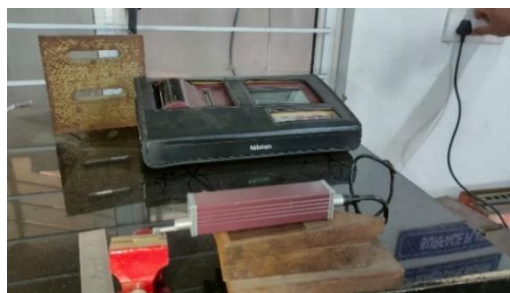
Fig. 4: Measuring Surface roughness of a machined sample of Nimonic alloy 75 by Mitutoyo surface tester
