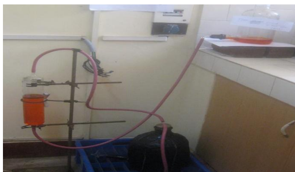
Fig. 1: Anaerobic Digester Setup.
