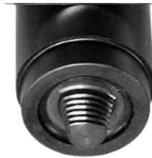
Fig. 7: Trivex tool, designed by TWI[27]
