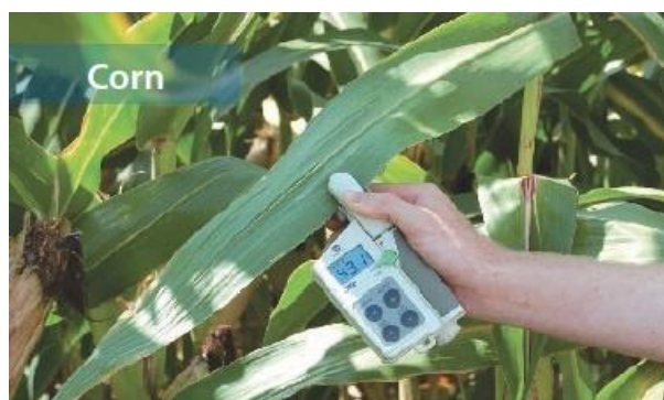
Fig. 4: A): Procedure for Using the Chlorophyll Meter.
