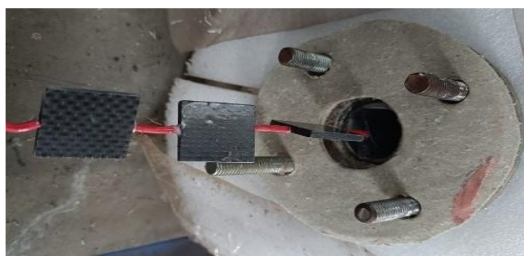
Fig. 4: Locating Inserts in the Test Section.
