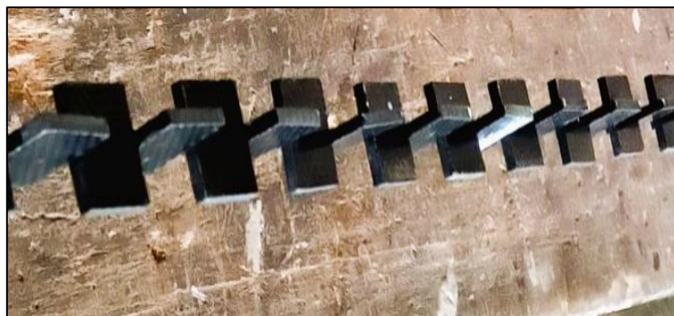
Fig. 3: Continuous Insert at 90° Twist Angle.
