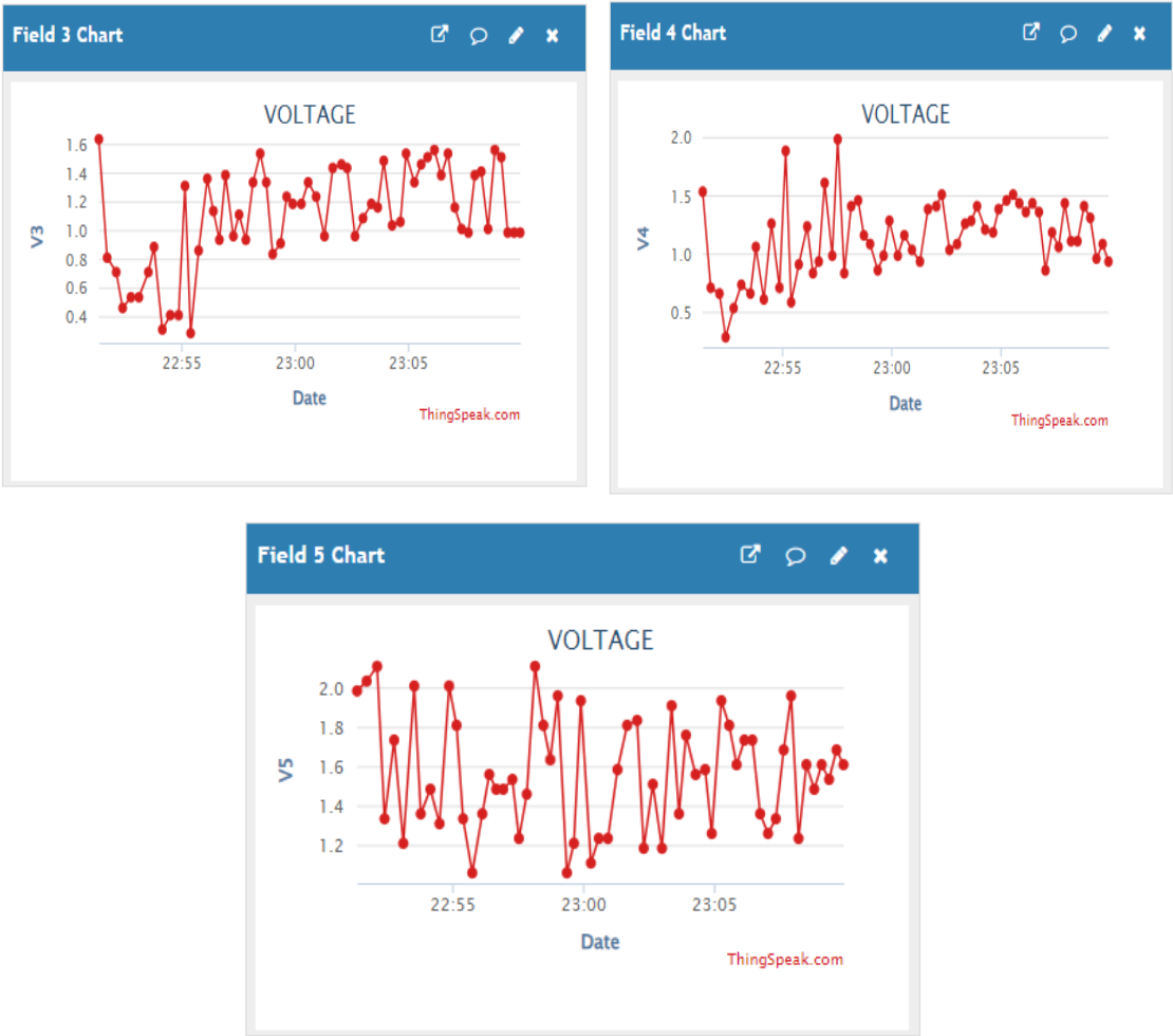
Fig. 4: Standalone solar PV output voltage in IoT Thing speak
