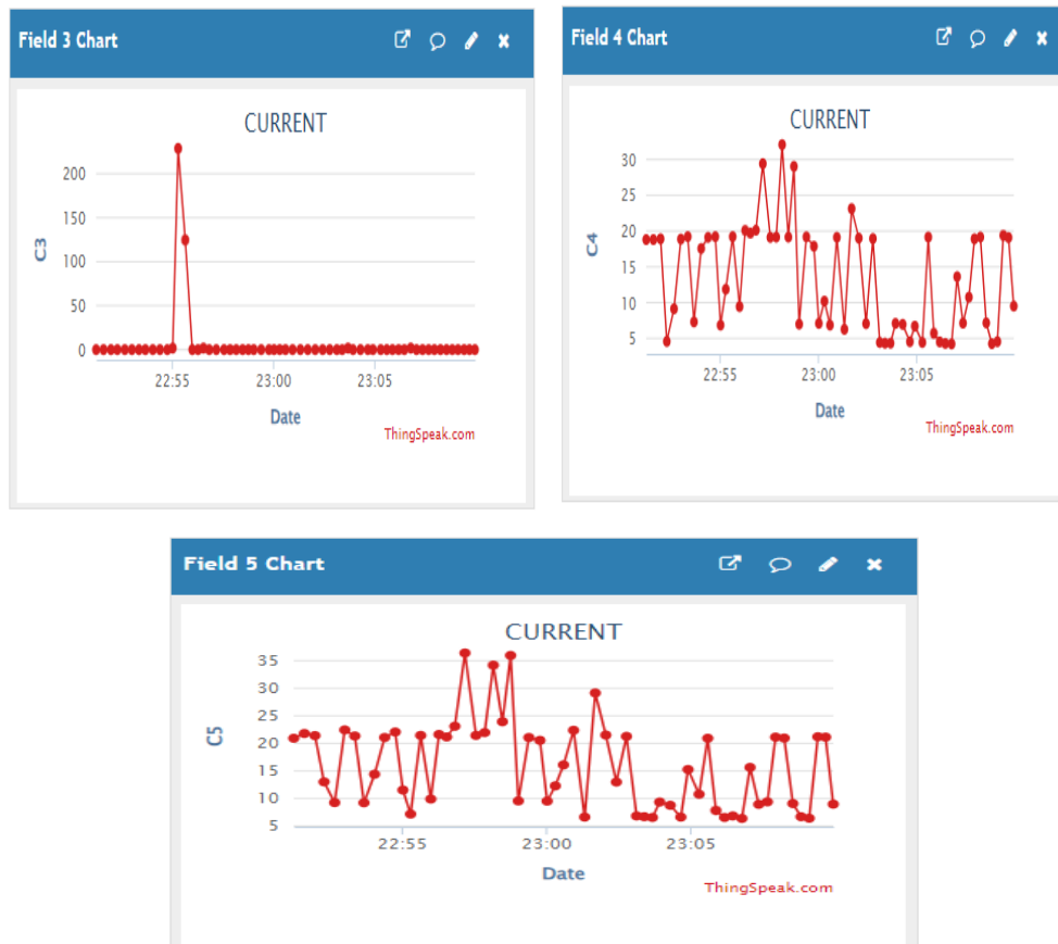
Fig. 5: Standalone solar PV output current in IoT Thing speak
