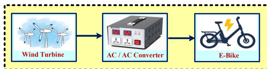
Fig. 2: Block Diagram of the Off-Grid Charging Station Powered by Wind Energy without Backup Battery.
