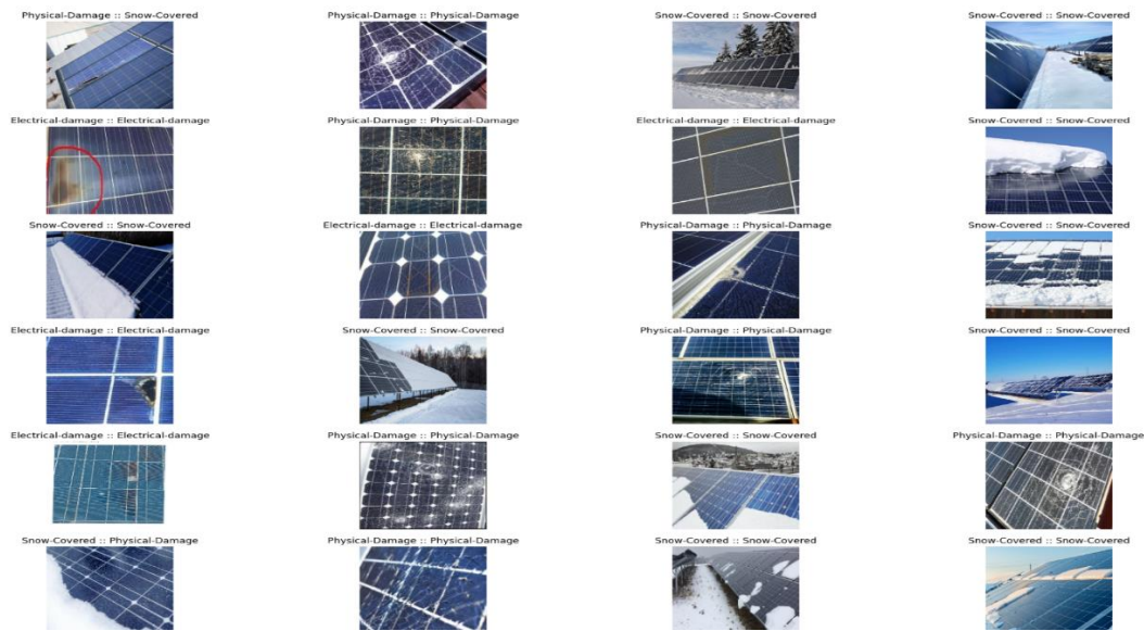
Fig. 4: Various Defects that occur in Solar Panel
