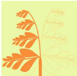
Fig. 3: Vivaldi Antipodal Antenna of Branches and Leaves.
