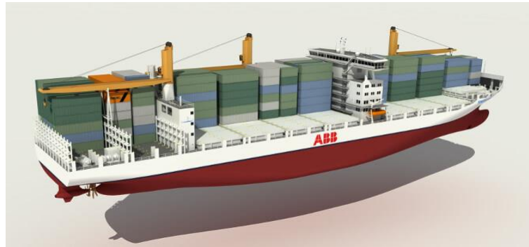
Fig. 2: 3D-Rendered Model of A Container Feeder Vessel, Specifically A 2000 TEU (Twenty-Foot Equivalent Unit) Class Ship. the Vessel Has A White and Red Hull with the Logo “ABB” on Its Side.
