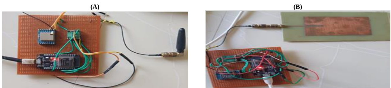
Fig. 12: A) ESP32 with 433Mhz RFM95W Lora, B) ESP32 with 866Mhz RFM95W Lora.
