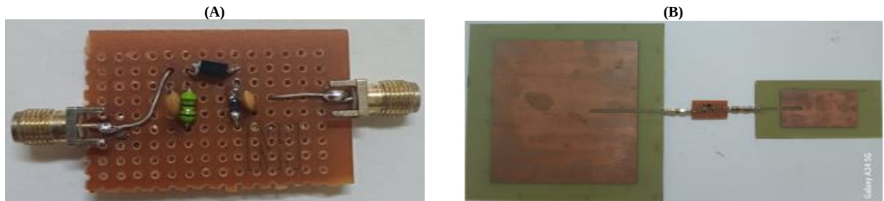
Fig. 11: Hardware Implementation of A) Frequency Doubler Using Schottky Diode, B) Frequency Doubling Reflectenna.
