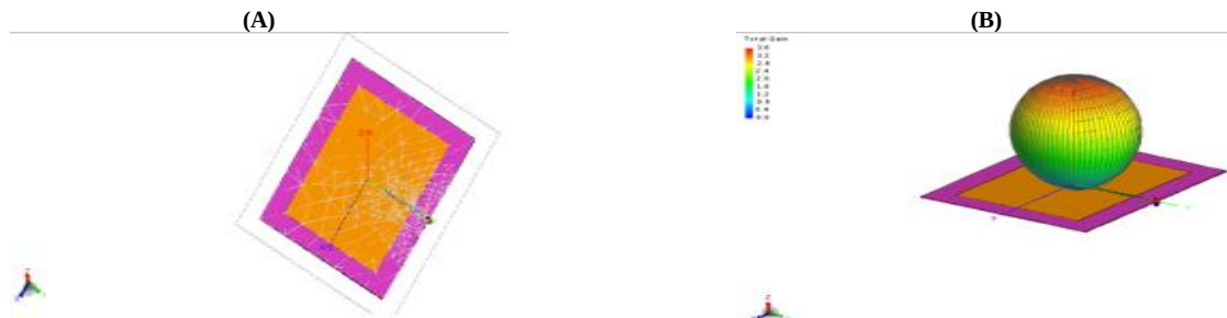
Fig. 4: A) Simulation of F1 Microstrip Antenna, B) Simulated Radiation Pattern and Gain of F1 Microstrip Antenna for 433 Mhz.
