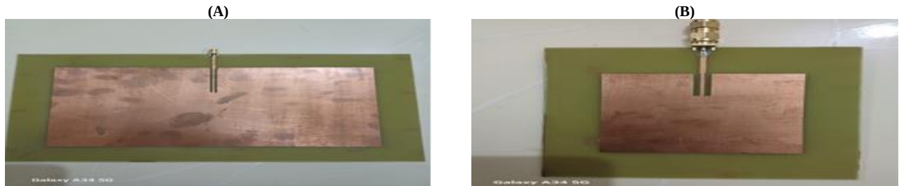
Fig. 10: Hardware Implementation of A) F1 Microstrip Antenna for 433 Mhz, B) Mf1 Microstrip Antenna for 866 Mhz.
