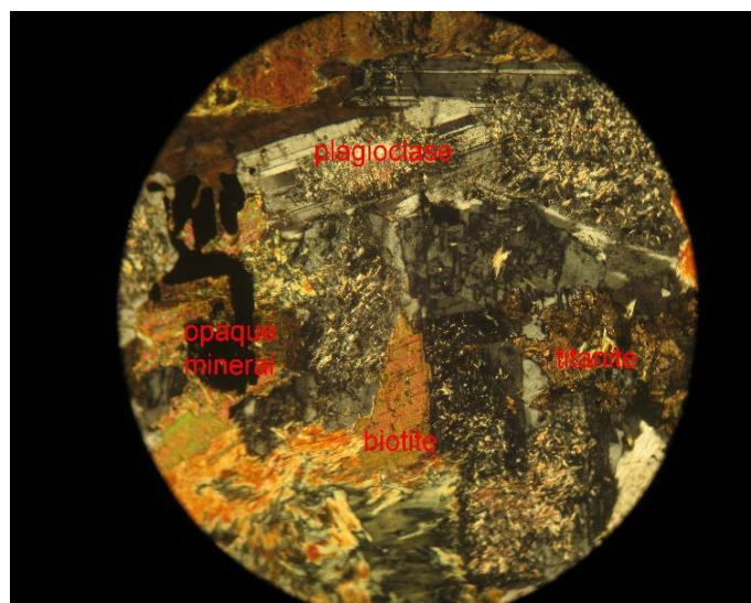
Fig. 11: Photomicrograph of Biotite Granite.
