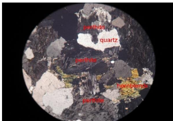
Fig. 14: Slide of Quartz-Feldspar Granite Porphyry.
