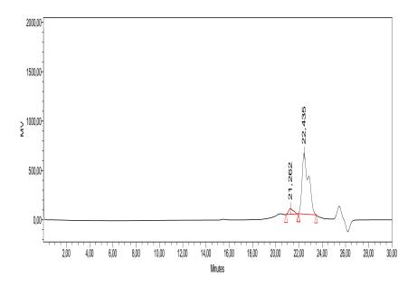
Fig 5: GPC chromatogram of PANI-ES with 6% Mag-H at  $0^{\circ}$ C for 1 h30 mn; Number-average molecular weight = 644 g/mol, weight-average molecular weight=746 g/mol, and Polydispersity=1.15.
