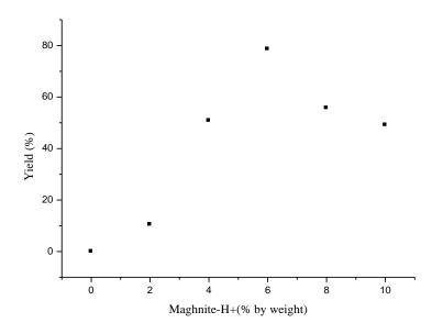
Fig. 8: Effect of the amount of Mag-H+ on the yield of the polymerization
