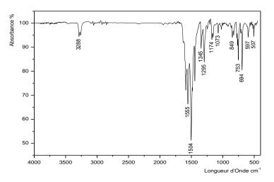
Fig. 1: Shows the characteristic FT-IR spectra of PANI-EB
