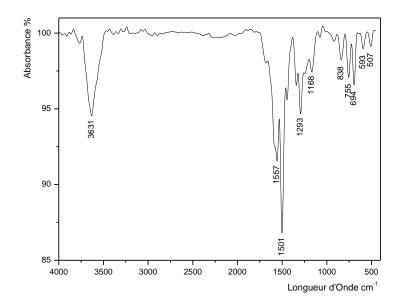
Fig.2: Shows the characteristic FT-IR spectra of PANI-ES
