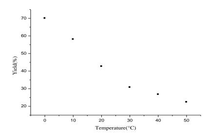
Fig. 9: Effect of the temperature on the yield of polyaniline (Maghnite-H+ = 6%, t=3h).
