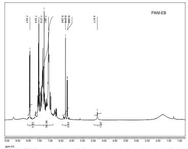
Fig. 4: 1H NMR spectrum (300 MHz, CDCl3, Tetramethylsilane (TMS) was used as the internal standard) of polyaniline (PANI-EB) obtained by the polymerization of aniline with Mag-H+ initiator system in CDCl3 at 25°C.
