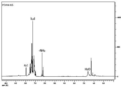
Fig. 3: 1H NMR spectrum (300 MHz, CDCl3, Tetramethylsilane (TMS) was used as the internal standard) of polyaniline (PANI-ES) obtained by the polymerization of aniline with Mag-H+ initiator system in CDCl3 at 0°C.
