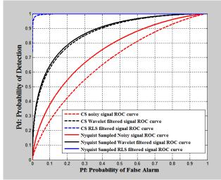
Fig. 8: Comparison between ROC Curves at 20% Compression Ratio and the Traditional Energy Detector Using Ordinary Sampling.
