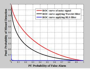
Fig. 6: Comparison Between ROC Curves for the Proposed Energy Detectors Based on De-Noising Filters and the Traditional Energy Detector Using Ordinary Sampling.
