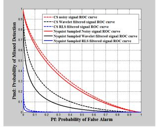
Fig. 13: Comparison between ROC Curves at 40% Compression Ratio and the Traditional Energy Detector Using Ordinary Sampling.
