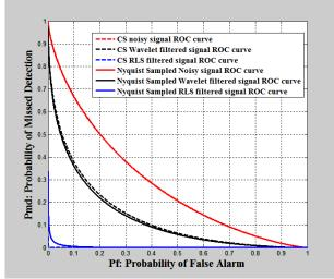
Fig. 15: Comparison between ROC Curves at 80% Compression Ratio and the Traditional Energy Detector Using Ordinary Sampling.
