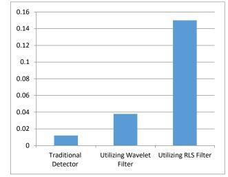
Fig. 7: Comparison between Throughputs for the Energy Detectors Based On De-Noising Filters and the Traditional Energy Detector Using Ordinary Sampling.
