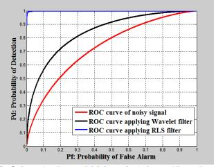
**Fig. 5:** Comparison Between ROC Curves for the Proposed Energy Detectors Based on De-Noising Filters and the Traditional Energy Detector Using Ordinary Sampling.
