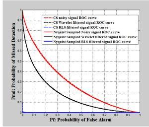
Fig. 14: Comparison between ROC at 60% Compression Ratio and the Traditional Energy Detector Using Ordinary Sampling.
