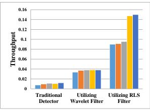
**Fig. 16:** Throughput Calculations for Traditional Energy Detector and the Proposed Energy Detectors Using Compressive Sensing at Different Compression Ratios.
