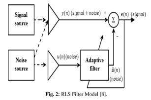
From Fig.2, two input signals y(n) and u(n) are applied simultaneously to an adaptive filter where, y(n) is a contaminated signal containing both uncorrelated desired signal s(n) and noise u(n). The main objective of the adaptive algorithm is to produce an optimum estimation of noise  $\hat{u}(n)$  in the contaminated signal. This can be achieved by using a suitable adaptive algorithm to minimize noise [20]. A simple equation of the RLS filter can be expressed as:
