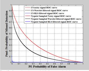
Fig. 18: Comparison between ROC Curves at Optimized Compression Ratio (64%) and the Traditional Energy Detector Using Ordinary Sampling.
