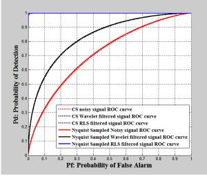
Fig. 10: Comparison between ROC Curves at 60% Compression Ratio and the Traditional Energy Detector Using Ordinary Sampling.
