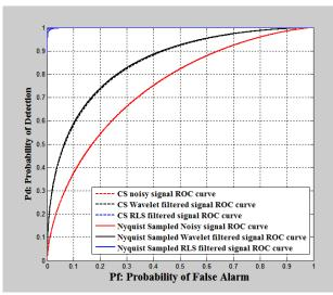
Fig. 17: Comparison between ROC Curves at Optimized Compression Ratio (64%) and the Traditional Energy Detector Using Ordinary Sampling.
