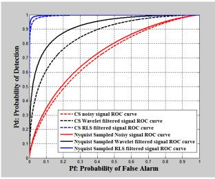
Fig. 9: Comparison between ROC Curves at 40% Compression Ratio and the Traditional Energy Detector Using Ordinary Sampling.
