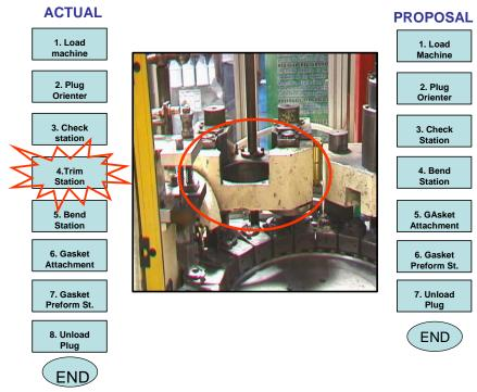
Fig. 15: Rengineering of the Process: Original (Left) vs. Proposed (Right) Methods, with A Photograph of the Trim Station (Center).
