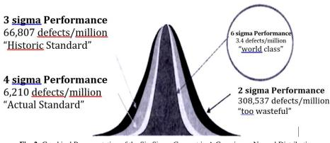
Fig. 2: Graphical Representation of the Six Sigma Concept in A Gaussian or Normal Distribution.
