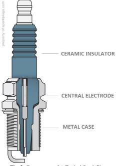
Fig. 3: Components of A Typical Spark Plug.
