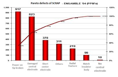
Fig. 5: Distribution of the Types of Defects in Spark Plugs.
