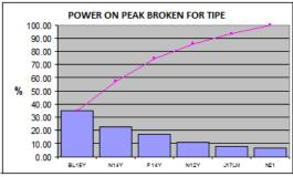
Fig. 7: Distribution of Broken Starting Tips per Each Type of Spark Plug.
