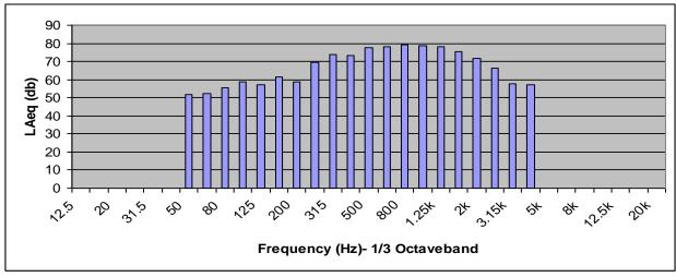
Fig. 3: The 1/3 Octave-Band Frequency Spectrum of the Equivalent Sound Pressure Level Measured at 600 M from the Main Blowdown.
