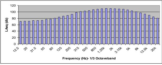
Fig. 2: The 1/3 Octave-Band Frequency Spectrum of the Equivalent Sound Pressure Level Measured at 80 M From the Main Blowdown.
