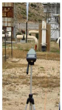
Fig. 1: The Photograph of the Sound Level Meter Used For the Measurements.
