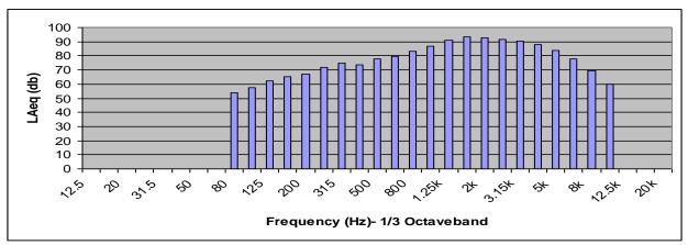
Fig. 4: The 1/3 Octave-Band Frequency Spectrum of the Equivalent Sound Pressure Level Measured at 25
