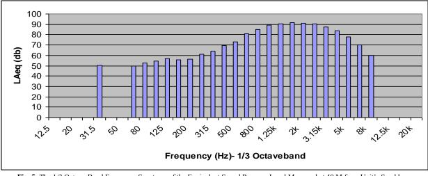
Fig. 5: The 1/3 Octave-Band Frequency Spectrum of the Equivalent Sound Pressure Level Measured at 40 M from Unit's Scrubbers.
