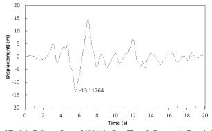
Fig. 16: Displacement of Upper Level of Tank in Fullness State of 100% in Case There Is Damper in Foundation Level Under Northridge Earthquake.
