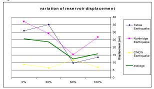
Fig. 11: Comparing Displacement of Upper Level of Tank in Empty Tank under the Studied Earthquakes
