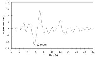
Fig. 17: Displacement of Upper Level of Tank in Fullness State of 100% in Case There Is Damper in Foundation Level Under Northridge Earthquake.
