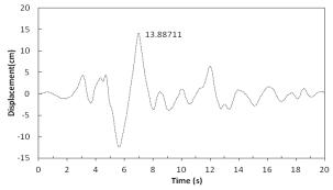
Fig. 13: Displacement of Upper Level of Tank in Fullness State of 100% in Case There Is Damper in Middle Level under Tabas Earthquake
