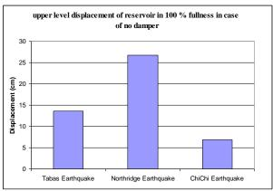
Fig. 6: Comparing Displacement of Upper Level of Tank in Fullness State of 100% under the Studied Earthquakes
