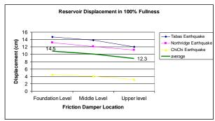
Fig. 25: Displacement of Upper Level of Tank in Fullness State of 100% for Different Positions of Damper.
