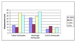
Fig. 10: Comparing Displacement of Upper Level of Tank in Empty Tank under the Studied Earthquakes
