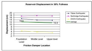
Fig. 29: Displacement of Upper Level of Tank in Fullness State of 30% for Different Positions of Damper
