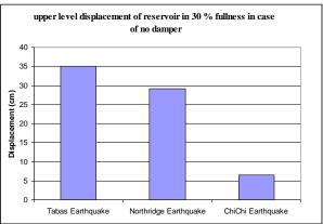
Fig. 8: Comparing Displacement of Upper Level of Tank in Fullness State of 30% under the Studied Earthquakes
