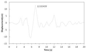
Fig. 14: Displacement of Upper Level of Tank in Fullness State Of 100% in Case There Is Damper in Upper Level under Tabas Earthquake
