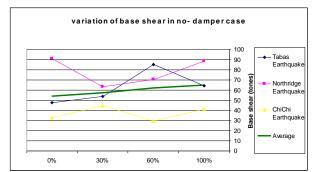
Fig. 35: Variations of Base Shear in Different States of Tank without Damper.
