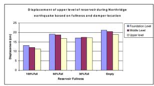
Fig. 33: Displacement of Upper Level of Tank Based on Position of Damper for Different States in Northridge Earthquake
