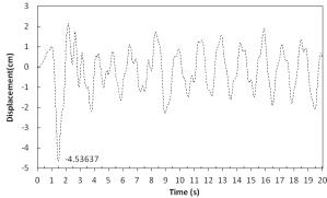
Fig. 20: Displacement of Upper Level of Tank in Fullness State of 100% in Case There Is Damper in Foundation Level Under Chi-Chi Earthquake.
