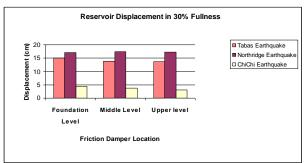
Fig. 28: Displacement of Upper Level of Tank in Fullness State of 30% for Different Positions of Damper
