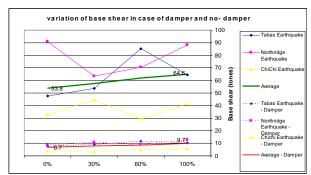
Fig. 37: Variations of Base Shear in Different States of Tank with or without Damper
