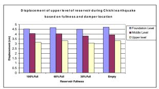
Fig. 34: Displacement of Upper Level of Tank Based on Position of Damper for Different States in Chi-Chi Earthquake
