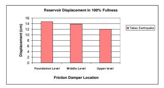
Fig. 15: Displacement of Upper Level of Tank in Fullness State of 100% for Different Positions of Damper under Tabas Earthquake
