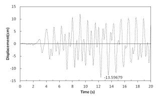
Fig. 3: Displacement of Upper Level of Tank in Fullness State Of 100% under Tabas Earthquake
