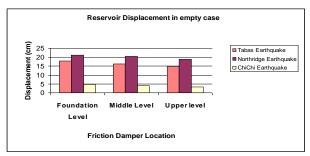
Fig. 30: Displacement of Upper Level of Empty Tank for Different Positions of Damper
