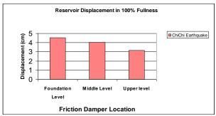
Fig. 23: Displacement of Upper Level of Tank in Fullnessstate of 100% for Different Positions of Damper Under Chi-Chi Earthquake
