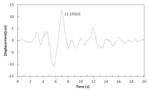
Fig. 18: Displacement of Upper Level of Tank in Fullness State of 100% In Case There Is Damper in Upper Level Under Northridge Earthquake.
