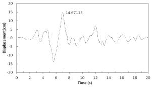
Fig. 12: Displacement of Upper Level of Tank in Fullness State Of 100% in Case There Is Damper in Foundation Level under Tabas Earthquake
