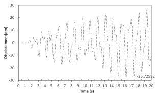
Fig. 4: Displacement of Upper Level of Tank in Fullness State of 100% under Northridge Earthquake.
