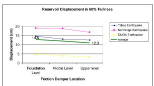
Fig. 27: Displacement of Upper Level of Tank in Fullness State of 60% for Different Positions of Damper.
