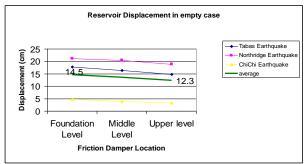
Fig. 31: Displacement of Upper Level of Empty Tank for Different Positions of Damper.
