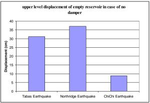
Fig. 9: Comparing Displacement of Upper Level of Tank in Empty Tank under the Studied Earthquakes
