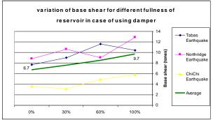
Fig. 36: Variations of Base Shear in Different States of Tank with Damper
