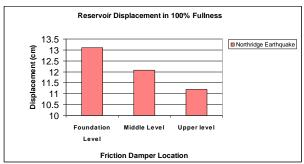
Fig. 19: Displacement of Upper Level of Tank in Fullness state of 100% For Different Positions of Damper under Northridge Earthquake
