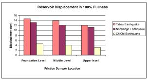
Fig. 24: Displacement of Upper Level of Tank in Fullness State of 100% for Different Positions of Damper
