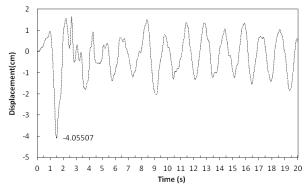
**Fig. 21:** Displacement of Upper Level of Tank in Fullness State of 100% in Case There Is Damper in Middle Level under Chi-Chi Earthquake Considering the above diagram, Displacement of middle level of tank in fullness state of 100% under Chi-Chi Earthquake is 4.0 cm in case there is damper in foundation level.
