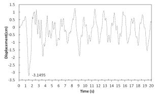
Fig. 22: Displacement of Upper Level of Tank in Fullness State of 100% in Case There Is Damper in Upper Level Under Chi-Chi Earthquake.
