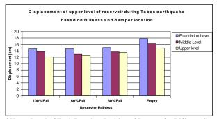
Fig. 32: Displacement of Upper Level of Tank Based on Position of Damper for Different States in Tabas Earthquake
