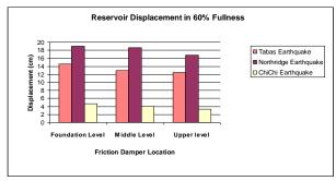
Fig. 26: Displacement of Upper Level of Tank in Fullness State Of 60% for Different Positions of Damper
