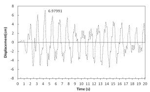
Fig. 5: Displacement of Upper Level of Tank in Fullness State of 100% under Chi-Chi Earthquake
