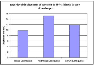
Fig. 7: Comparing Displacement of Upper Level of Tank in Fullness State of 60% under the Studied Earthquakes
