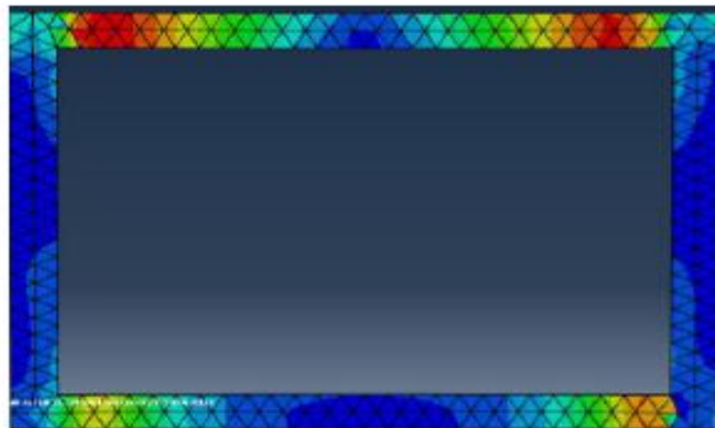
Fig. 13: Stress Contour in Hard Soil
