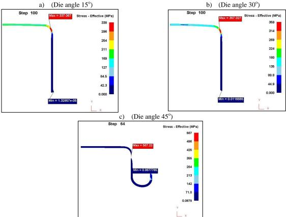
Fig. 12: Stress Distribution on the Product (Cup) According to Die Cone Angle
