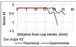
Fig. 10: Distribution of thickness strain for three cases
