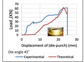
Fig. 8: Load Displacement Relationship of (Die-Punch) for Three Cases
