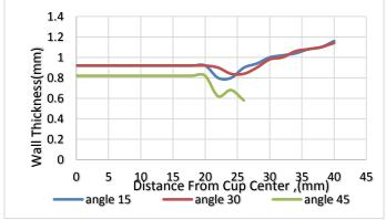
Fig. 9: Experimentally Wall Thickness Distribution of the Cup
