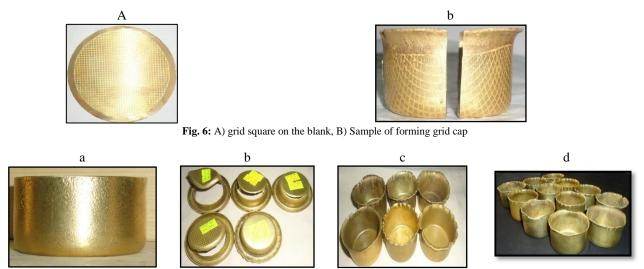
Fig. 7: Samples of Drawen Cups A) Completed Successful Cup, (B,C &D) Cups Produced with Die of Con Angle 45°,15° and 30° Respectively
