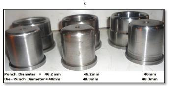
Fig. 4: A) Assembly of Rig B) Dies Geometry C) Punches and (Die-Punches)
