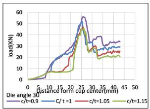
Fig. 11: Drawing Load Clearance Ratio Relationship
