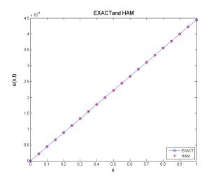
**Fig. 3:** Shows the Comparison between Exact and (HAM) t=0.9,  $\hbar=-1$
