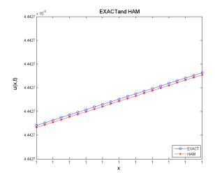
**Fig. 4:** Zoom For Comparison between Exact and (HAM) Solutions At 0.9999999999  $\le x \le 1$ , t = 0.9,  $\hbar = -1$
